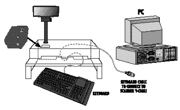
Thread **Keyboard Cable** through **right front slot** of **Cash Drawer Shoe** and out through **back slot** of **Cash Drawer Shoe**. Place **Keyboard** on lower "shelf."
