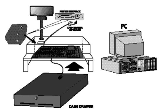
Thread Cash Drawer Cable up through *rectangular slot on top* of Cash Drawer Shoe and connect to the *back* of the Receipt Printer, as shown in illustration. Slide Cash Drawer under Cash Drawer Shoe, and align front of drawer with front of Cash Drawer Shoe.
