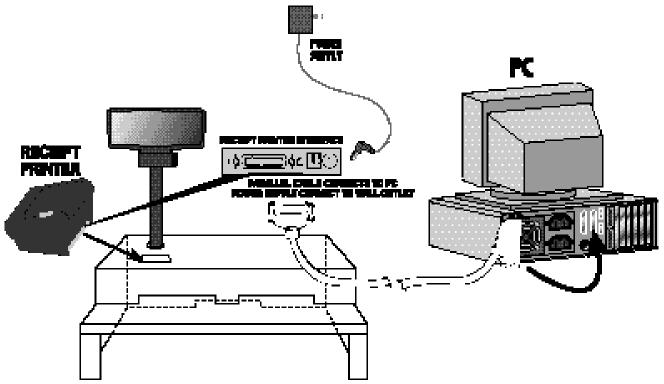
Thread both **Parallel Cable** and **Power Supply Cable** up through **rectangular slot** on top of **Cash Drawer Shoe** (in front of Pole Display) and connect to **back** of **Receipt Printer**. Thread other ends of **Parallel Cable** and **Power Supply** out through **back slot** of **Cash Drawer Shoe**. Connect **Parallel Cable** to **Parallel Port** on back of your PC, and plug **Power Supply** into standard wall outlet.
